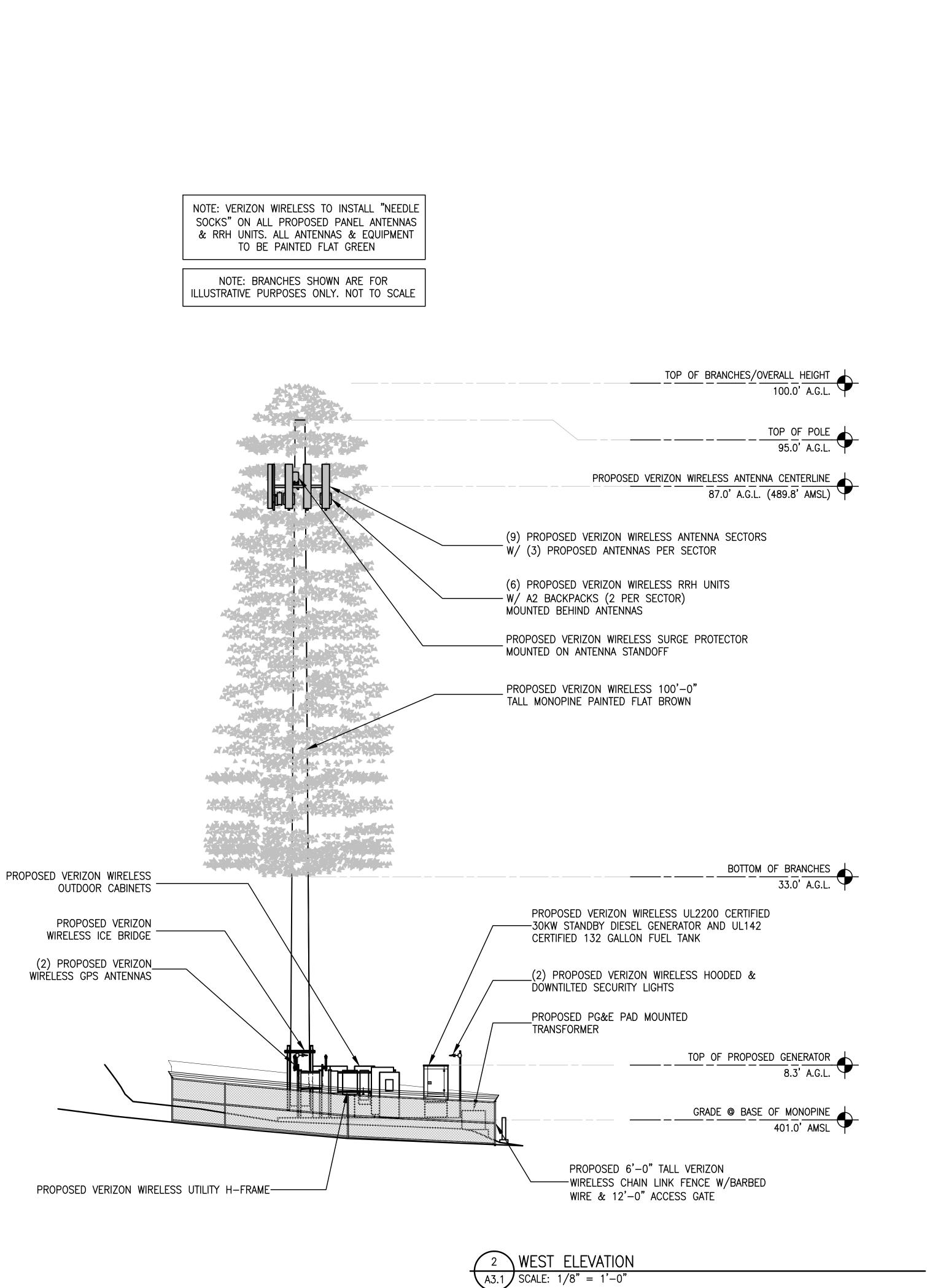
NOTE: VERIZON WIRELESS TO INSTALL "NEEDLE SOCKS" ON ALL PROPOSED PANEL ANTENNAS & RRH UNITS. ALL ANTENNAS & EQUIPMENT TO BE PAINTED FLAT GREEN
