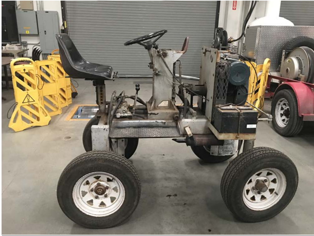
Image: weight cart- used to move up to 3-1,000-pound weight blocks
