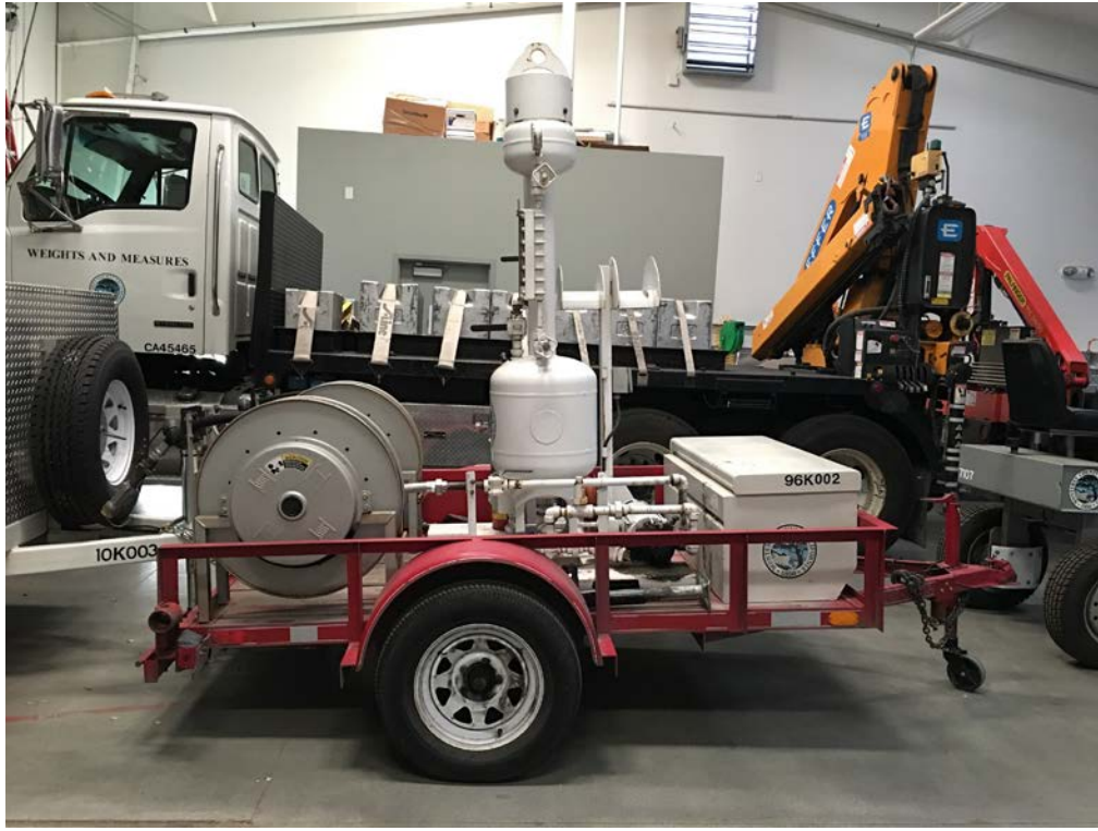
Image: 20-gallon LPG prover on a trailer – certified test standard used to test retail LPG meters
