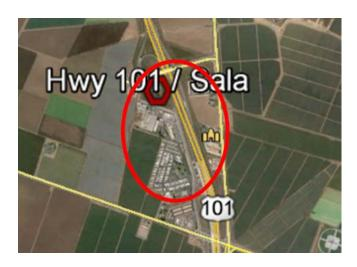
The search ring represents the area within which a facility can be located to produce the desired coverage objective. The centerline height of 60' represents the required height of the antennas to produce the desired coverage objective.
