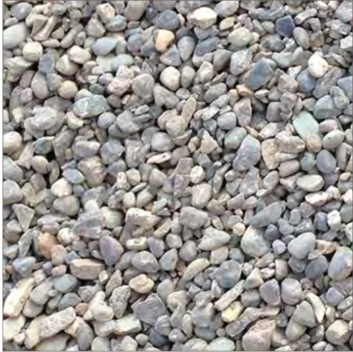
5 #3 ROOFING BALLAST- 1'-2" LARGE ROUNDED RIVER ROCK; WHITE AND LIGHT-GRAY COLOR
