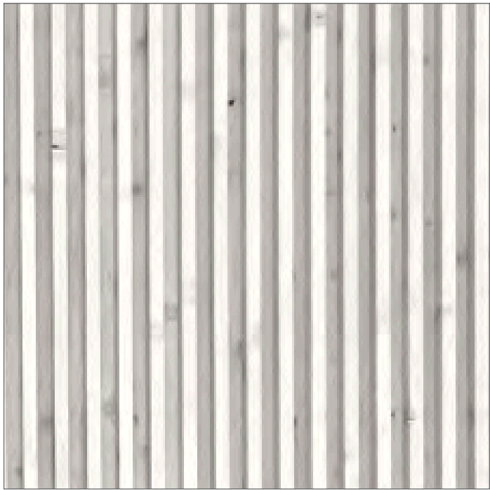
1 VERTICAL BOARD & BATTEN WOOD CLADDING - 2X2 BATTENS SPACED EVERY 4" O.C.; WHITE-WASH FINISH
