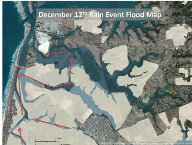
Figure 14. Comparison of Modeled 100-year flow paths and observed flow paths during Dec 2014 flood (Figure source: ESA 2014)
