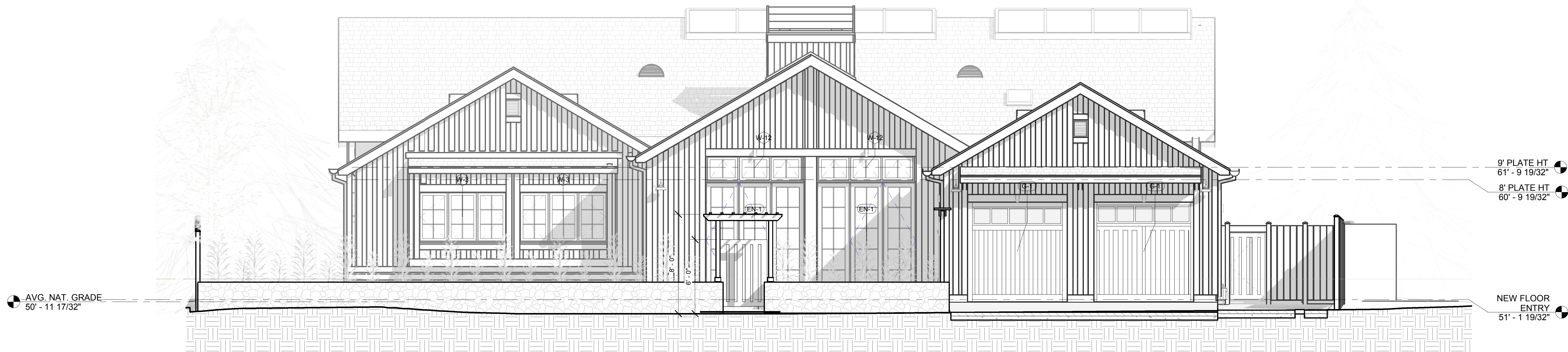
1 PROPOSED SOUTH ELEVATION SCALE: 1/4" = 1'-0"
