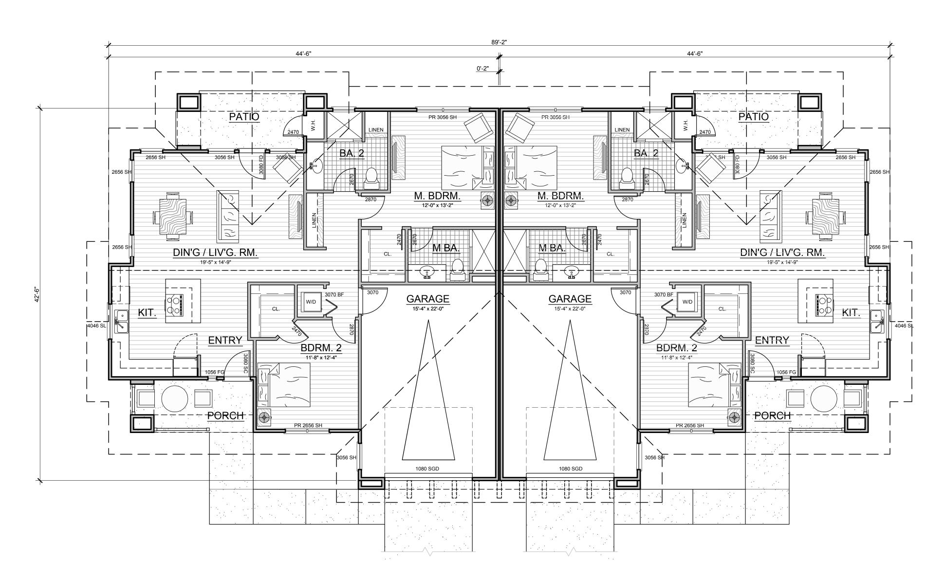
BUILDING COORDINATION PLAN - BUILDING TYPE 3 - B / B UNITS SCALE 3/16" = 1'-0"
