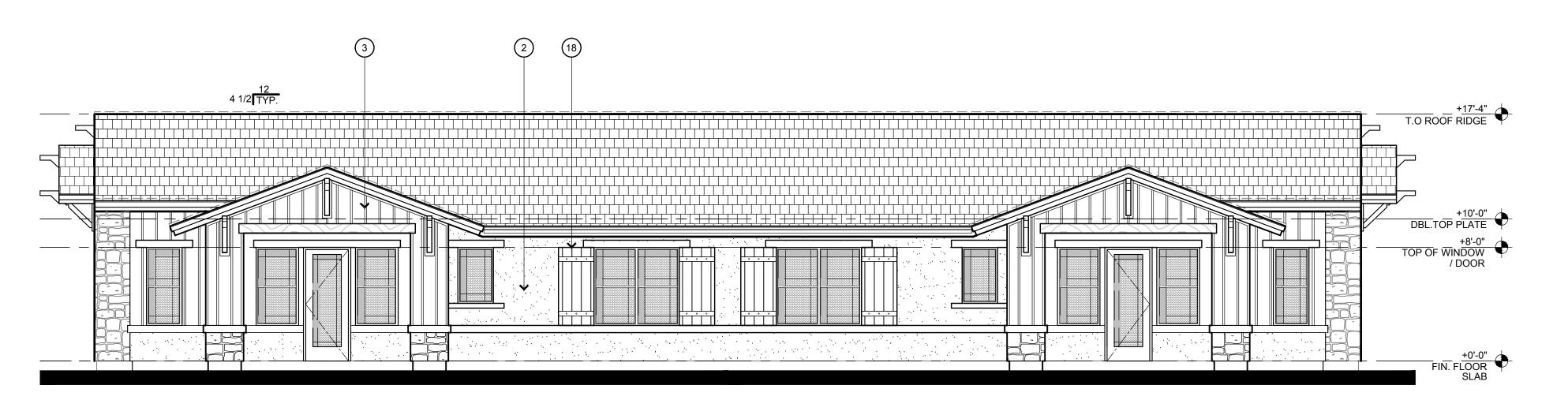
REAR ELEVATION - BUILDING TYPE 3 - B / B UNITS SCALE 3/16" = 1'-0"
