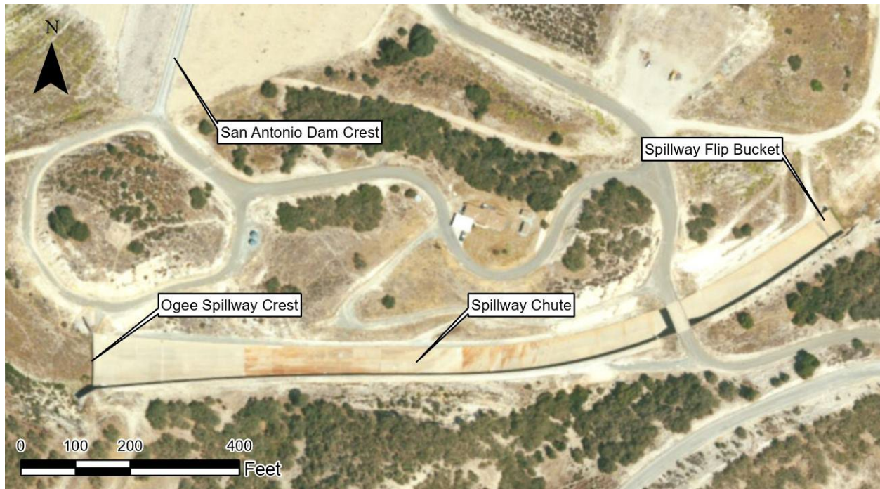
Figure 2: San Antonio Dam Spillway Alignment
