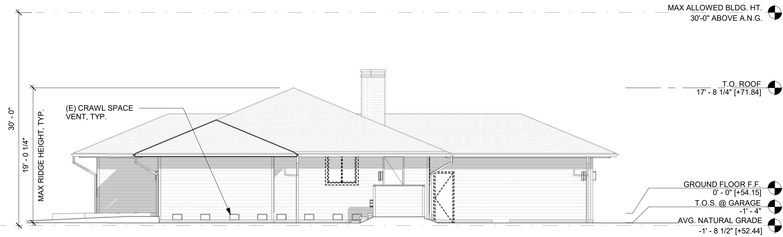
EXISTING EAST EXTERIOR ELEVATION 1/8" = 1'-0" 3
