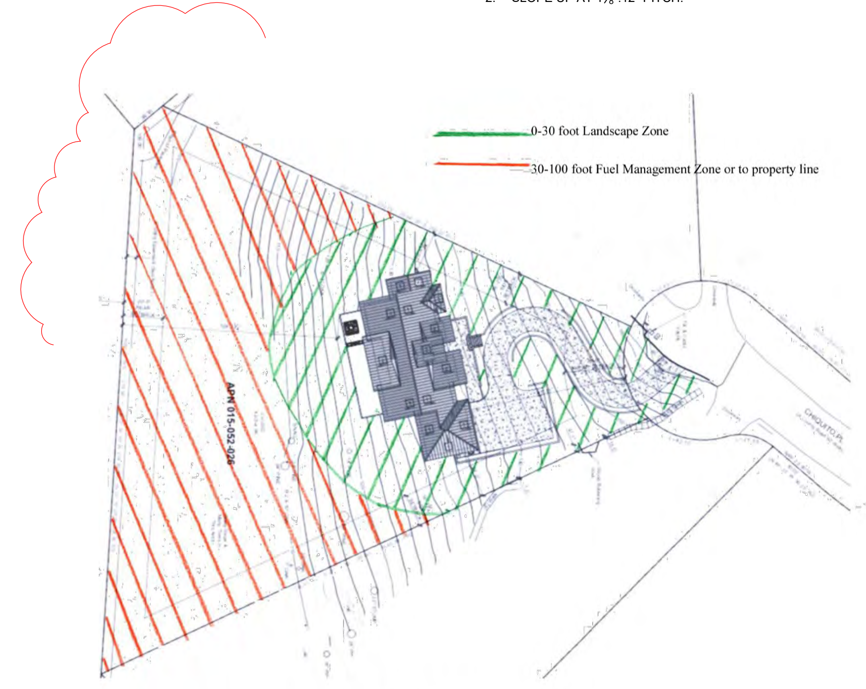
Exhibit A: Fuel Management Zone map. The 0-30 foot Landscape Zone around the proposed home is approximate and is identified in green, and the approximate 30-100+ ft area identified in red is the Fuel Management Zone, or also commonly referred to as the Reduced Fuel Zone and Defensible Space Zone.
