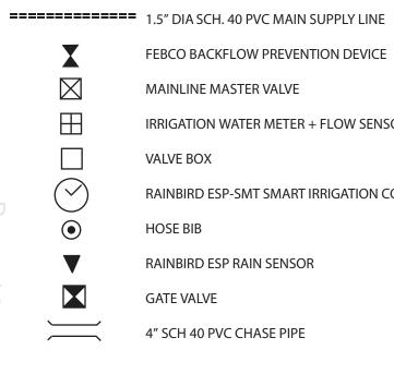
FEBCO BACKFLOW PREVENTION DEVICE MAINLINE MASTER VALVE IRRIGATION WATER METER + FLOW SENSOR VALVE BOX RAINBIRD ESP-SMT SMART IRRIGATION CONTROLLER HOSE BIB RAINBIRD ESP RAIN SENSOR GATE VALVE 4" SCH 40 PVC CHASE PIPE
