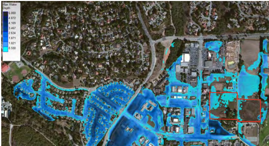
Figure 4. CSA-50 Report illustrating ponding/flooding depths through the CSA area. Project site shown in red.
