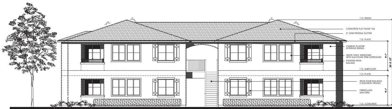
Front/Rear Elevation- Two Story Elevation
