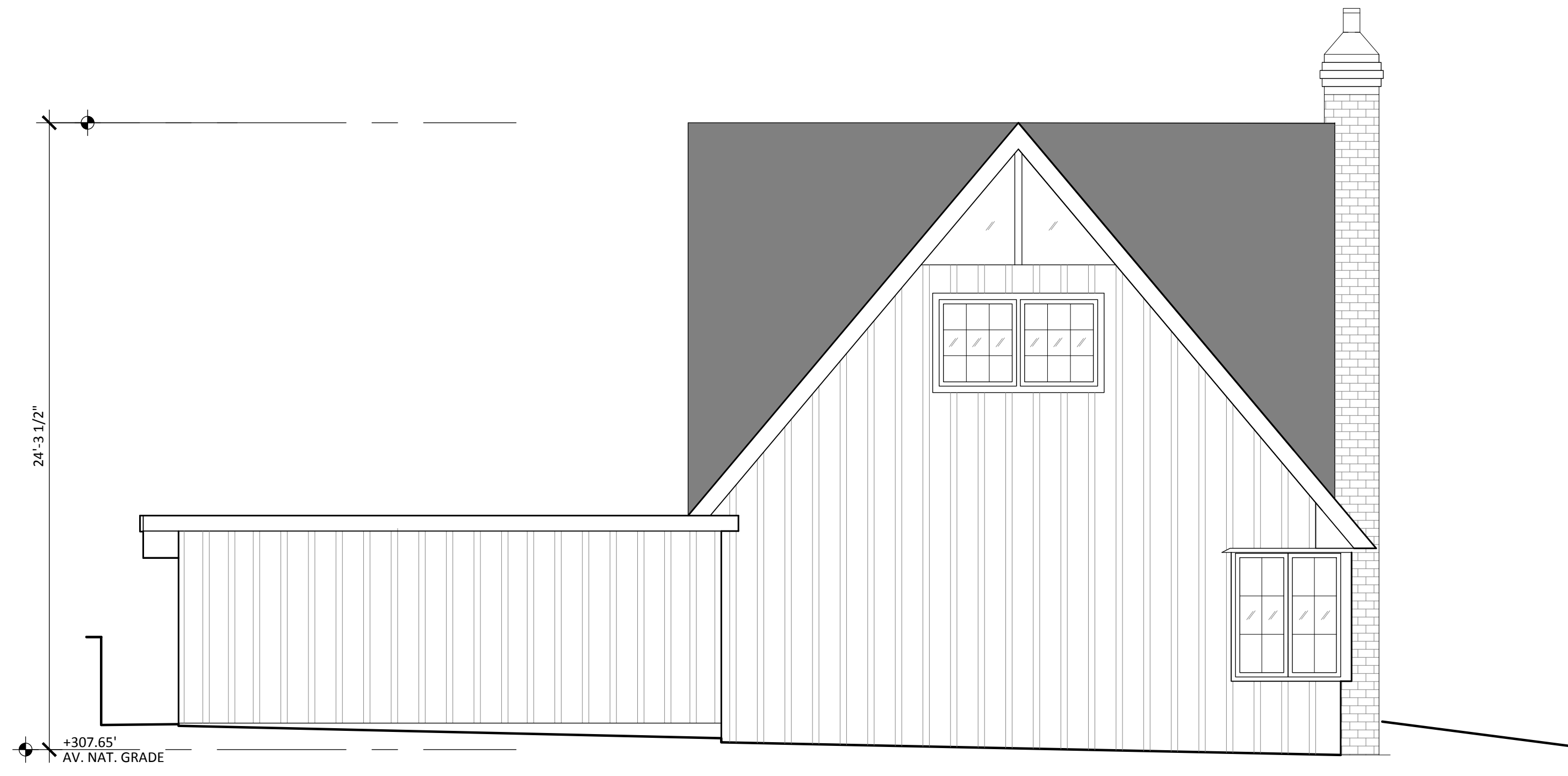
1 EXISTING ELEVATION- EAST 1/4"=1'-0"
