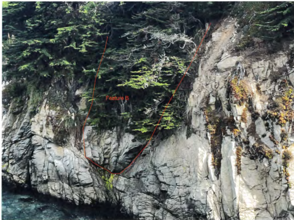
Feature B – Potential Wedge Failure.
