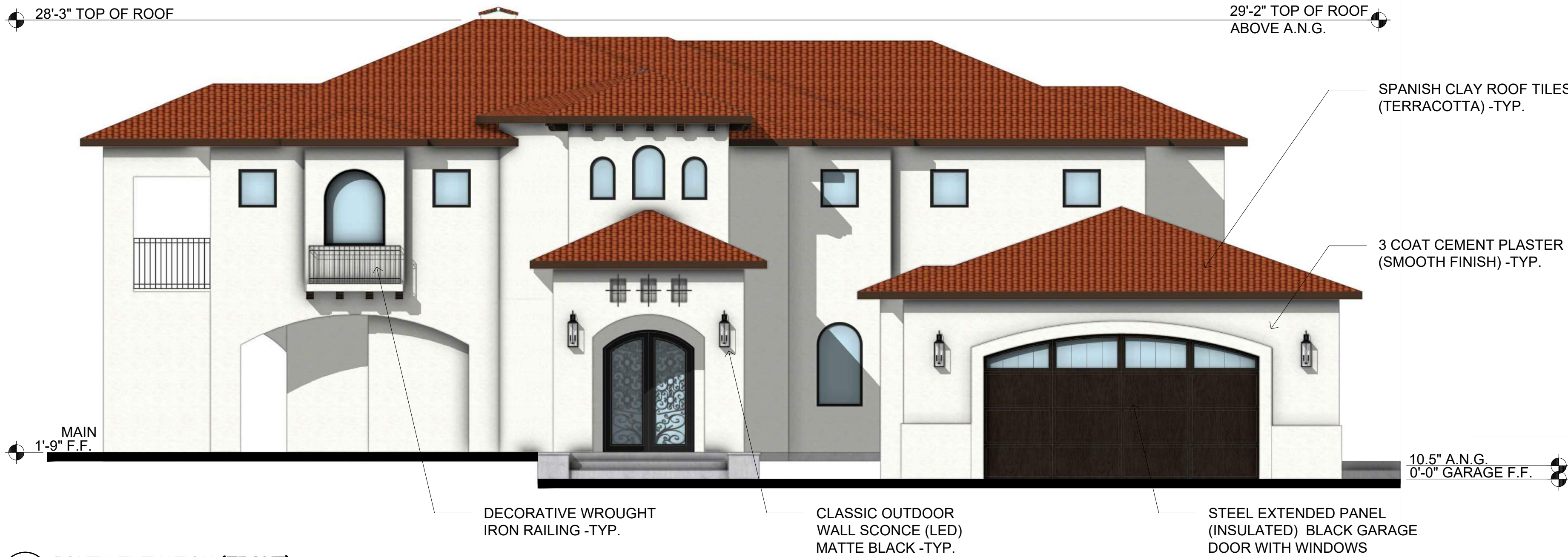
1 SOUTH ELEVATION (FRONT) SCALE: 3/16" = 1'-0"
